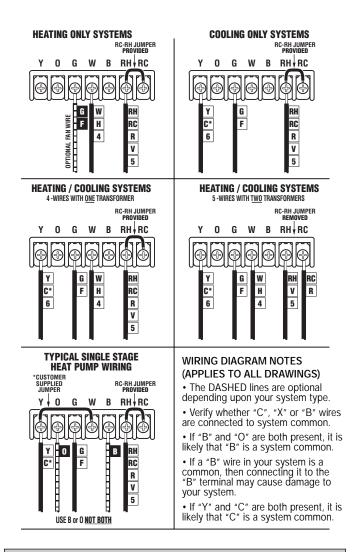
These diagrams below are provided for new installations or unreferenced wires.
